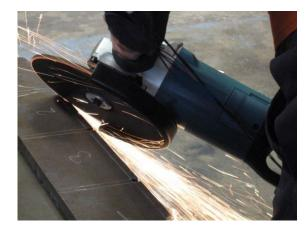
Hand-held angle grinders are widely used across a number of sectors, including steel frame fabrication. Grinders typically produce noise levels of around  $L_{Aeq}$  90 – 95 dB(A), so are significant contributors to occupational noise exposure.
